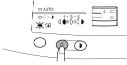
Press the exposure mode selector key twice. The photo (in) indicator will stop blinking and the AUTO indicator will light up steadily. The toner save mode is now active.
